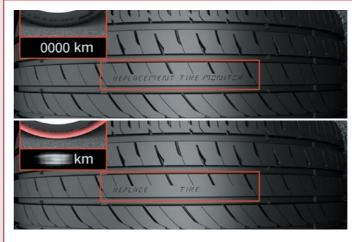
The RTM (Replacement Tire Monitor) provides the vehicle owner with added safety by clearly indicating when the tyres need to be replaced.
